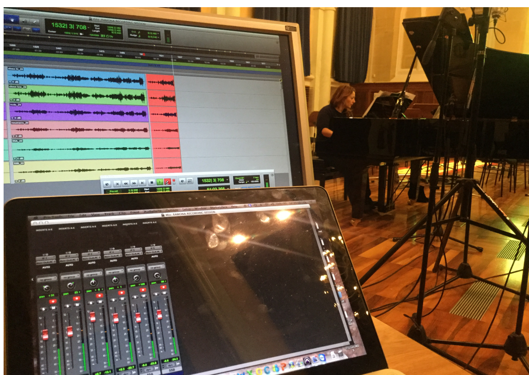
Plate 16: Recording moment during Piano Pastels showing the six simultaneous microphones input signals being fed in Pro Tools which included a close matched pair, MS configuration and an XY setup 5/6 feet away from the piano. Pianist Ramona Zammit Formosa is seen behind the monitor screens during the recording.
