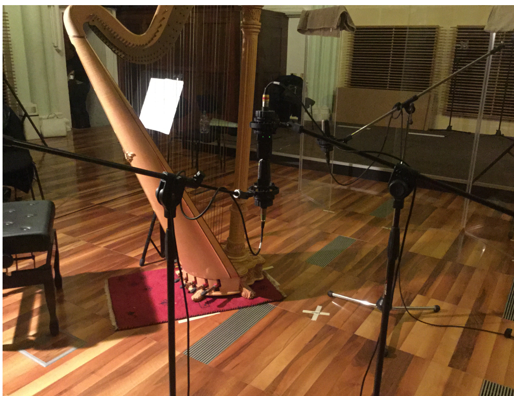
Plate 12: The XY Microphone setup for the harp using a matched pair of AKG 414s. An extra spot microphone was placed on one side directed towards the sounding box.
