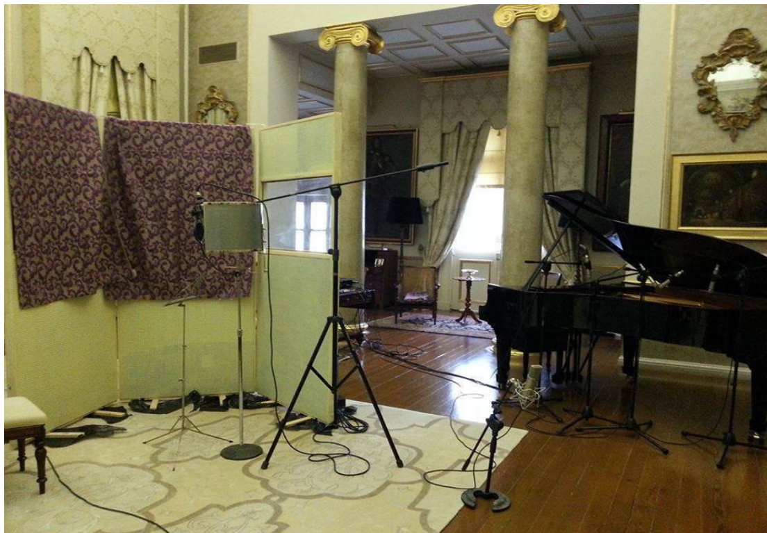
Plate 6: The recording set-up at the Malta President's Grand Masters' Hall. The Neumann U87 microphone on the bottom right shows the position where the cellist was placed.
